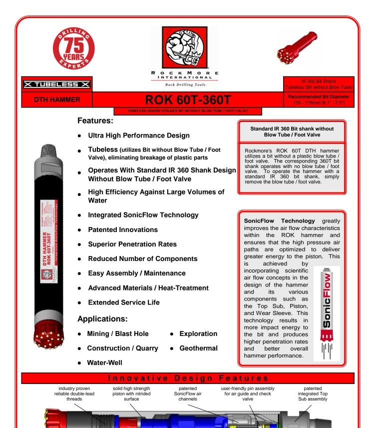
360T tubeless shank (standard IR 360 shank without blow tube), 8 spline design
