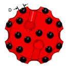
FEWER, LARGER DIAMETER **CARBIDE RESULTS** IN SLOWER PENETRATION RATES. BUT LONGER CARBIDE AND BIT LIFE.
